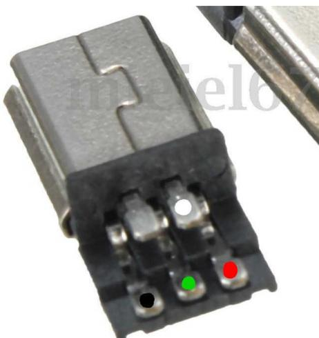
All you really have to do is to match the cable colours to the tabs on the USB connector in the picture above. **Make sure NONE of the tabs are touching each other, or that there is solder connecting them together. Don't guess that its ok, make 100% sure, or it can damage things – your PC, the teensy, etc.**
