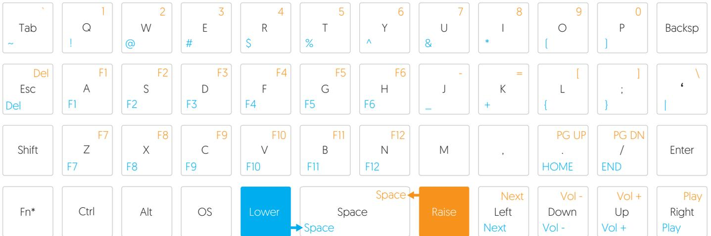
\* Fn presses shift and cycles through the backlight settings
